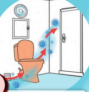
If toilet has not been used for long time or occupants forget to pour water into the floor drain regularly, the water seal in the trap can evaporate gradually and lose its capability to prevent foul odour or unclean substances from entering the premises
